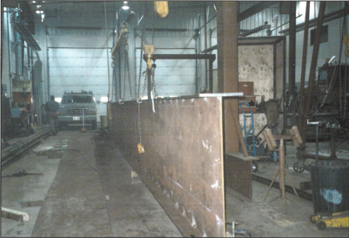
Figure 1 Fit-up of main girder.
